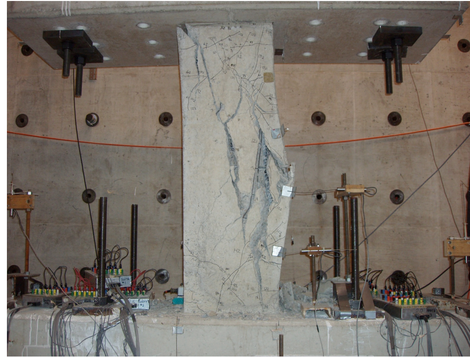
Purdue 1 after axial failure
